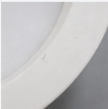
Photo 4. Example minor scratches in the white trim finish.
