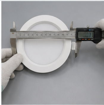
Photo 7. Example trim diameter measurement using a digital caliper.
